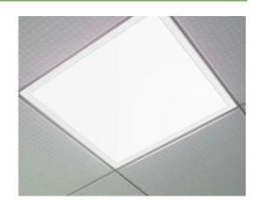
The Stratosphere II High Output Selectable Panel is 5-wattage and 5-CCT selectable, replacing up to 25 dedicated wattage & CCT models. It is backlit for higher efficiency, and easily installs recessed or surface mounted. A built-in junction box fits standard T-grid ceilings. The housing is constructed of a white aluminum heat sink, with a high transmittance polycarbonate lens that never yellows. These panels are both cULus and DLC listed.
