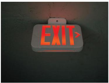
The Red White Exit Sign is a durable emergency exit sign. It provides 1W of red LED backlight output for the classic red letter exit sign design. The battery backup provides more than 90 minutes of emergency operation for safe building egress and code compliance. The 5W input wattage recharges the unit within 24 hours of battery backup use. Mounting options include back-to-wall mount, side-to-wall mount, or top-to-ceiling mount.
