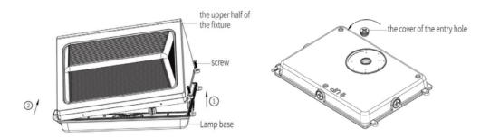
3. Punch holes in the lamp base that correspond to the embedded junction box.
